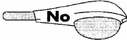
light trespass and excessive lighting (MCC 3.14). All exterior lighting should use full cutoff luminaires with the light source downcast and fully shielded (see illustration below).
