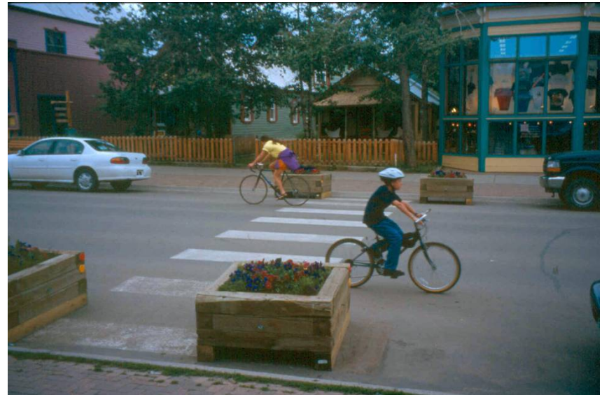
Figure 43: Summer curb extensions, Crested Butte
