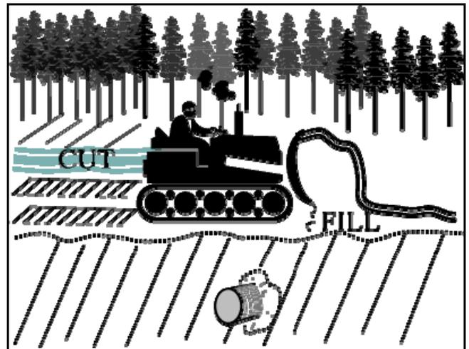
Forest roads are often built by excavating the road surface out of a hillside. A bulldozer starts at the top of the cut slope, excavating and sidecasting material until the desired road width is obtained.
