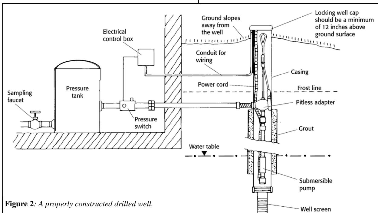
**Figure 2:** A properly constructed drilled well.
